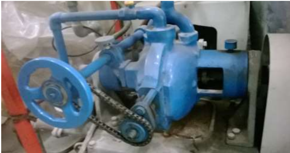
Figure 3.1: Water Brake Dynamometer
