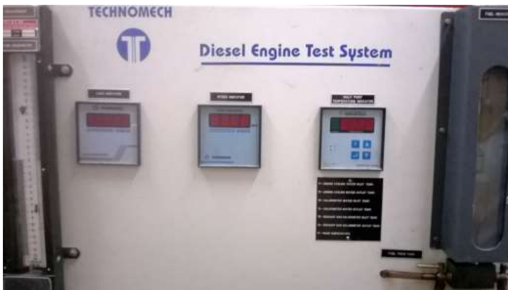
Figure 2.2: Temperature, Load and Speed indicator
